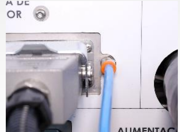
Water hose (steam generator)
