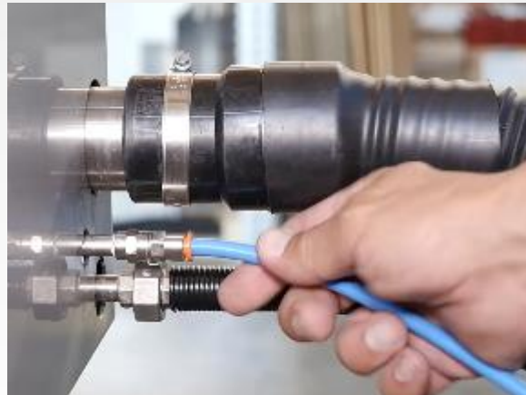
Water hose (belt cleaning head)
